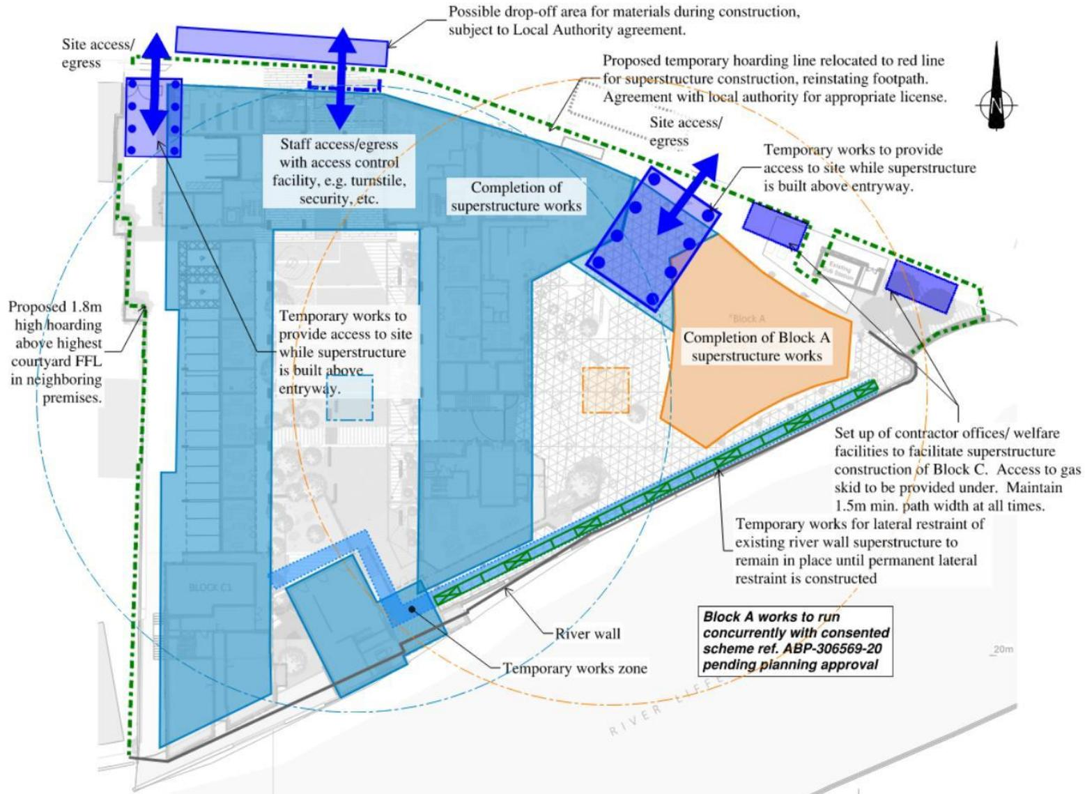
Figure 4.7 Overall sequencing of Works (6 of 7)
