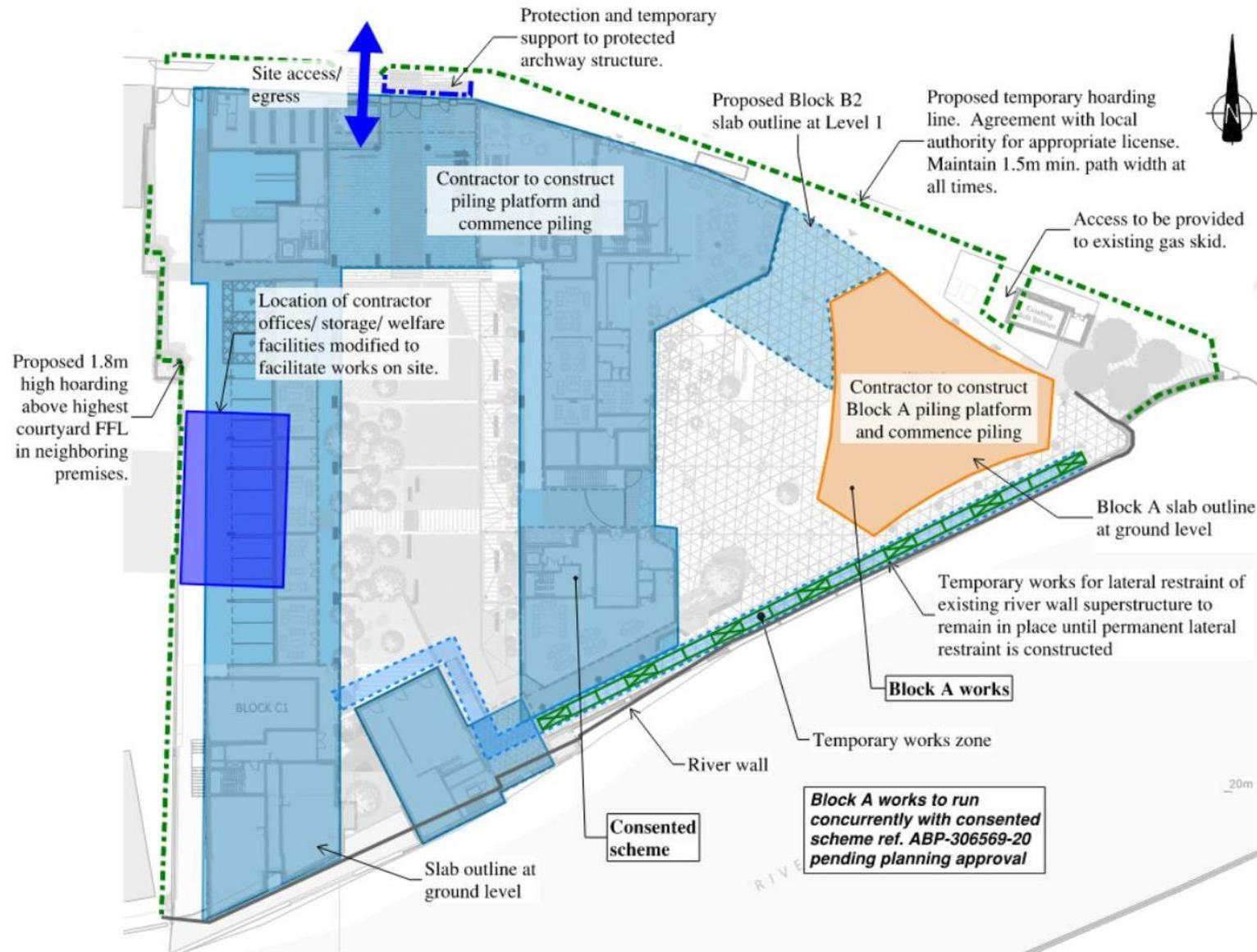
**Figure 4.3** Overall sequencing of Works (2 of 7)
