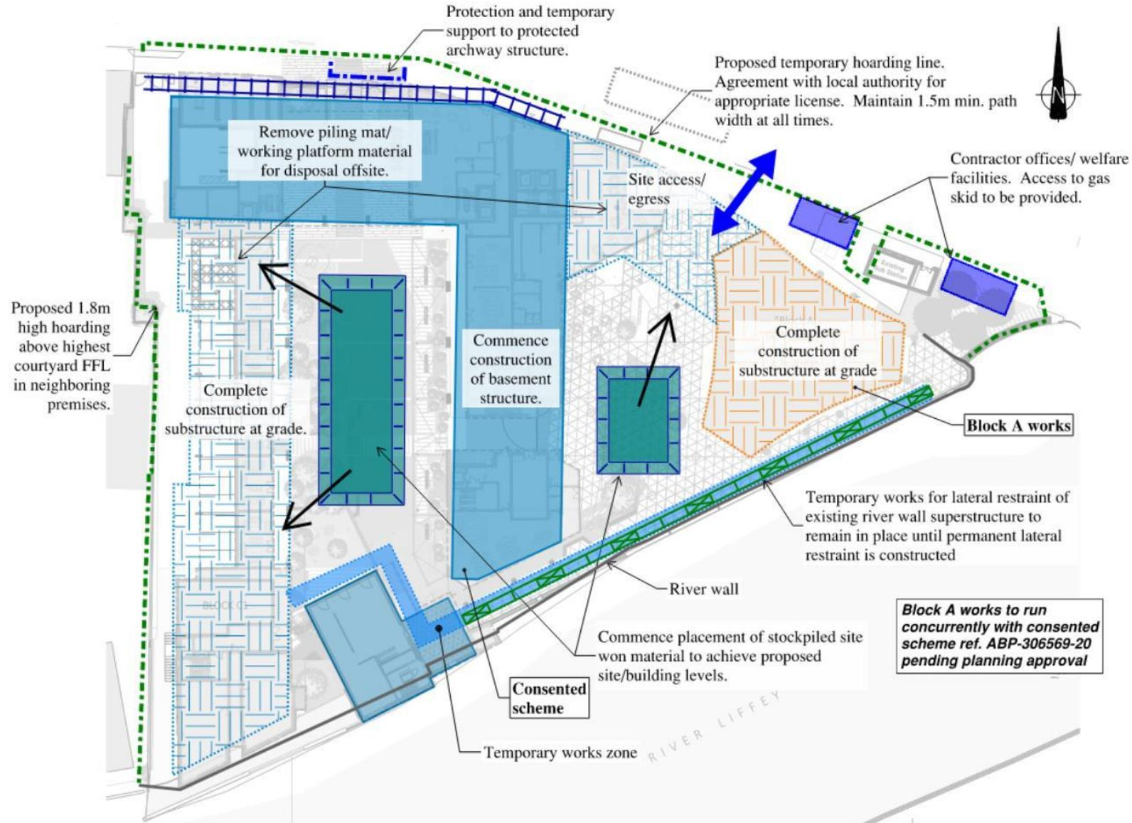
**Figure 4.5** Overall sequencing of Works (4 of 7)
