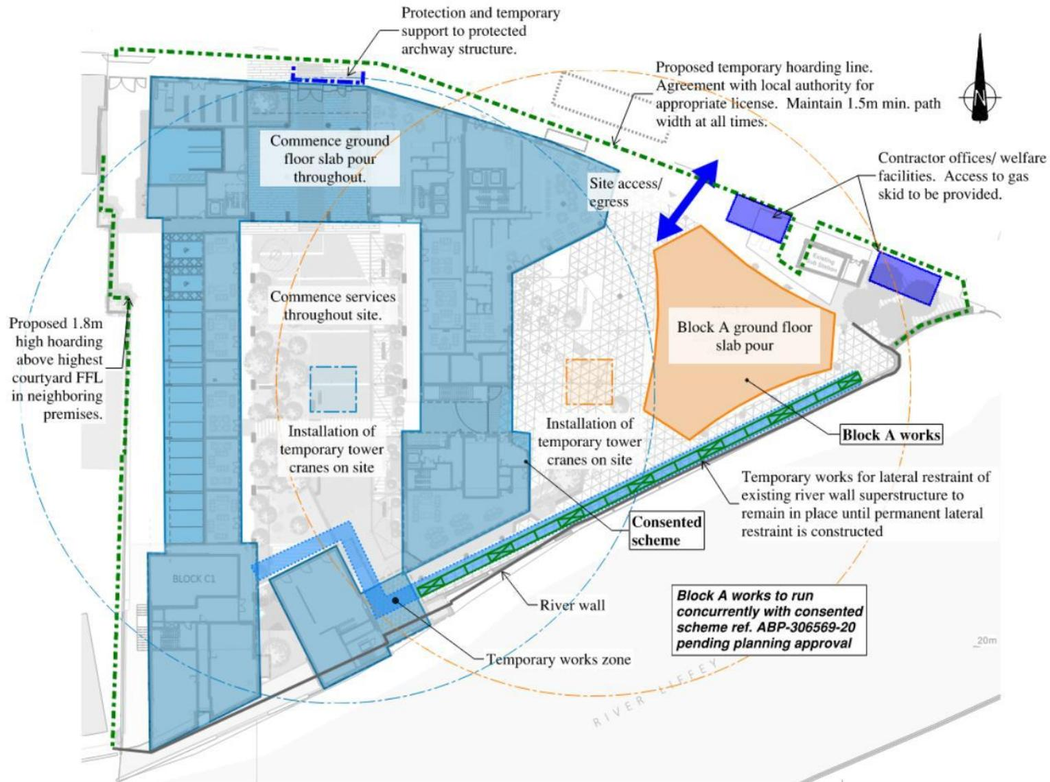
**Figure 4.6** Overall sequencing of Works (5 of 7)
